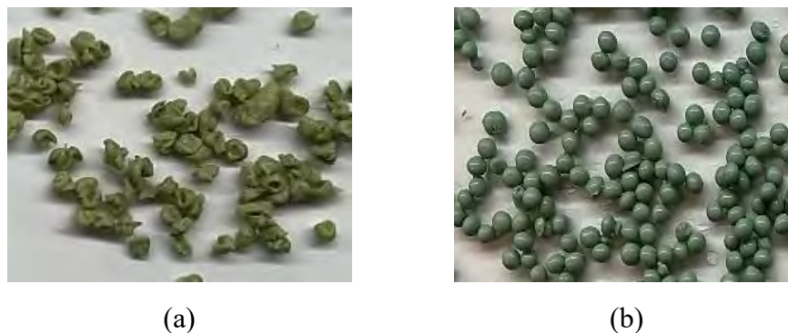
Fig. 2 – Zeolite NaX (a) and Saccharomyces cerevisiae yeast (b) immobilized in alginate after sorption of copper ions from solution with an initial concentration of 9.825 \text{ mmol L}^{-1}
