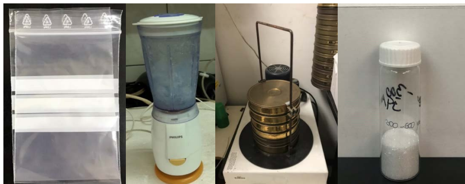
Slika 2. Postupak pripreme LDPE mikroplastike Figure 2. Procedure for preparation of LDPE microplastics
