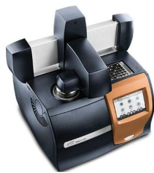
**Description of the method:** DSC is a method of thermal analysis of the samples that allows the user to determine Glass Transition of the samples, Heat Capacity (cp), onset and peak temperatures of phase transitions (e.g. crystallization), kinetics, oxidation induction Time (OIT).
