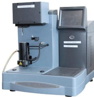
**Description of the method:** TGA is an analytical method that monitors the change in mass of a sample as a function of temperature or time. TGA can be non-isothermal, when the temperature changes linearly with time, or isothermal, when the temperature to which the sample is heated is constant. Thermograms enable determining the sample thermal stability at different temperatures and the composition of multiphase systems.
