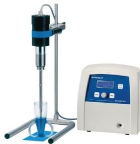
**Description of the method:** Ultrasonic homogenizer known as a sonicator uses high-frequency sound waves to disrupt cells or tissues. It works by creating high-energy sound waves in a liquid medium, which causes a phenomenon called cavitation.
