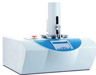
**Description of the method:** Differential scanning calorimetry (DSC) is a thermal method in which the analyzed and reference sample are heated at equal heating rates, and the heat required to maintain both samples at the same temperature, regardless of the changes occurring in the test sample, is measured. The method enables the determination of physical and chemical changes of the sample that occur under the influence of heat (phase transitions or reactions in which enthalpy changes occur).
