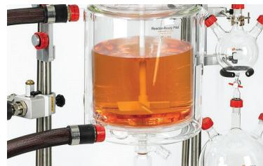
**Technical description of the device:** Reactors are glass vessels of different sizes and volumes, with several inlets. The inlets on the reactor can be used to connect the necessary devices for monitoring the reaction (e.g., oxygen electrode, pH electrode...) and for the feeding of the reaction mixture.
