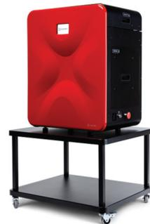
**Description of the method:** Selective laser sintering is a 3D printing technology that uses polymer powder as a starting material. The powder is applied in a thin layer on the build platform by means of a mechanism and melted with a laser to obtain the finished object.
