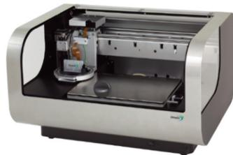
**Description of the method:** Inkjet printing technology is based on the ejection of ink in the form of droplets from the nozzles of the tank under piezoelectric effect. Due to gravity and air resistance, the droplet is projected onto the substrate in a certain position. This is a non-contact digital printing technology that produces fine structures of 30 micrometers and less
