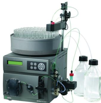
**Description of the method:** Fast protein liquid chromatography (FPLC), is a form of liquid chromatography that is often used to analyze or purify mixtures of proteins. As in other forms of chromatography, separation is possible because the different components of a mixture have different affinities for two materials, a moving fluid (the mobile phase, an aqueous solution or buffer) and a porous solid (the stationary phase, resin composed of beads of varying sizes and surface ligands).
