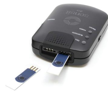
**Description of the method:** The Sensit BT is ideal for electrochemical sensor applications. The Sensit BT connects via Bluetooth to smartphone or tablet and controlled via the Android app PStouch. You can use the USB-C port to charge the Sensit BT or connect to a classic USB port on your PC and control the Sensit BT via our PC software PSTrace. The Sensit BT supports most common electrochemical techniques, including Cyclic Voltammetry, Square Wave Voltammetry and Impedance Spectroscopy.
