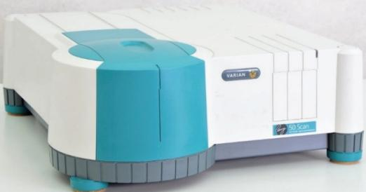
**Description of the method:** A spectrophotometer is employed to measure the amount of light that a sample absorbs. It operates by passing a beam of light through a sample and measuring the intensity of light reaching a detector. When a photon collides with an analyte molecule, its absorption can occur, which depends on the analyte structure and photon energy (wavelength). This absorption reduces the number of photons in the beam of light, thereby reducing the intensity.
