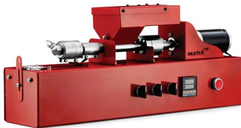
**Description of the method:** The single-screw extruder is used to produce polymer or composite filament with a thickness of 1.75 mm or 3.00 mm from material resin.
