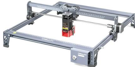
**Description of the method:** The laser engraver uses a 10 W laser, which it directs using 6 lenses, to engrave or cut various materials with high precision.
