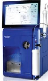
**Description of the method:** Column chromatography (CC) is a method of separating the components of a mixture consisting of a stationary and mobile phases. The stationary phase is a solid adsorbent, usually silica gel, and the mobile phase is a solvent or solvent mixture. The separation of the components depends on the binding strength of the substance to the adsorbent and on the substance solubility in the mobile phase. The obtained UV spectra confirm the purity of the mixture components.
