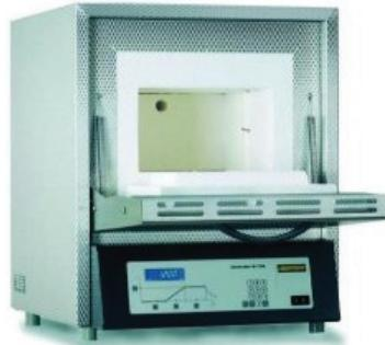
**Technical description of the device:** The volume of the furnace is 5 L. The furnace has a power of 2.4 kW. It does not have built-in ventilation, i.e. drainage of gases formed during heating of the samples.
