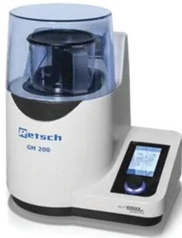
**Description of the method:** The Knife Mill is suitable for the rapid and reproducible size reduction and homogenisation of samples.
