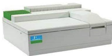
**Description of the method:** Analytical spectroscopic methods are based on measurement of the radiation amount reflected or absorbed by atomic or molecular species in the sample. When sample is exposed to the beam of light, there is a decrease in the intensity of the output radiation that is measured. This phenomenon is called light absorbance and is equal to the logarithm of the ratio of incoming and outgoing radiation.
