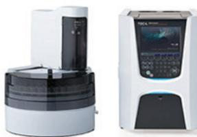
**Description of the method:** TOC analyzers use the catalytic oxidation method by burning at a temperature of 680°C. This method enables efficient oxidation of a wide range of compounds, covering concentrations from 4 µg/L to 30,000 mg/L, with an extremely low detection limit of 4 µg/L. Catalytic oxidation combustion allows the oxidation of both easily degradable low molecular weight organic compounds and difficult-to-degrade, insoluble, and macromolecular organic compounds.
