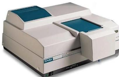
**Description of the method:** A spectrophotometer measures the amount of light absorbed by a sample. A beam of light is passed through the sample, and the intensity of the light that reached the detector is measured. The obtained data provide information about the structure of the materials that make up the sample.
