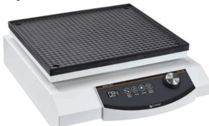
**Description of the method:** The unique, modular system allows simultaneous mixing, shaking and tempering without the need for an additional warming cabinet.
