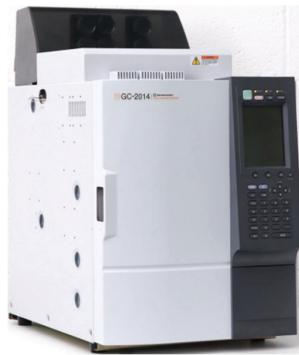
**Description of the method:** Gas chromatography (GC) is an analytical technique that uses gas as a mobile phase and sample is heated up and vaporized. Each compound of sample can be separated and quantified.
