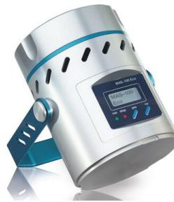
**Description of the method:** The instrument draws air through a perforated plate with a high performance suction device. The particle-bearing airflow is directed onto a standard Petri dish containing agar. On completion of the collection cycle, the Petri dish is incubated and the total colony count determined.
