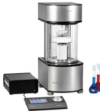
**Description of the method:** Tensiometer is used to measure the density and surface tension of liquid, and interfacial tension between two liquids. The method measures the mass, where a metal ring, plate, or holder with cylinder is attached to the weighing system of the tensiometer. Surface tension and interfacial energy are calculated based on the measured max. force when slowly withdrawing the ring or plate from the liquid. Density is calculated based on the measured buoyancy force.
