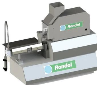
**Description of the method:** Extrusion is a process of continuous preforming in which molten material is forced through a die, whereupon the extruded material hardens by cooling with water or air to form an extrudate, i.e., a continuous/semi-finished product with a specific thickness and width.
