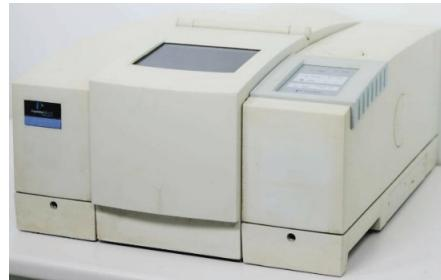
**Description of the method:** FT-IR is a technique for identification and characterization of different inorganic and organic samples. It is based on the interaction of infrared (IR) radiation with the sample. Absorption of IR radiation occurs at such wavelengths (energies), which correspond to the energies of vibrations of the atoms in the sample (depending on the bond type and on characteristic groups in the structure of the sample).
