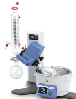
**Description of the method:** Rotary evaporation is the process of reducing the volume of a solvent by distributing it as a thin film across the interior of a vessel at elevated temperature and reduced pressure. This promotes the rapid removal of excess solvent from less volatile samples.
