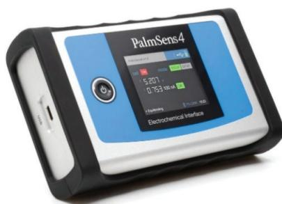
**Description of the method:** PalmSens4 is a USB and battery powered Potentiostat, Galvanostat, and optional a Frequency Response Analyser (FRA) for Electrochemical Impedance Spectroscopy (EIS). PalmSens4 has a large potential range (-5V to 5V or -10V to 10V) and current range (100 pA to 10 mA) with a high resolution and low noise. PalmSens4 is a complete laboratory instrument but also ideal for field work. Connecting via Bluetooth guarantees a perfectly floating measurement.
