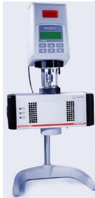
**Description of the method:** The RheolabQC is a rotational rheometer which works according to the Searle principle. It consists of a highprecision encoder and a highly dynamic EC motor. You can select between controlled shear rate (CR) and controlled shear stress (CS) test settings. These options, together with the wide speed and torque ranges and very short motor response times, bring innumerable benefits for the application. As well as conventional flow and viscosity curves.
