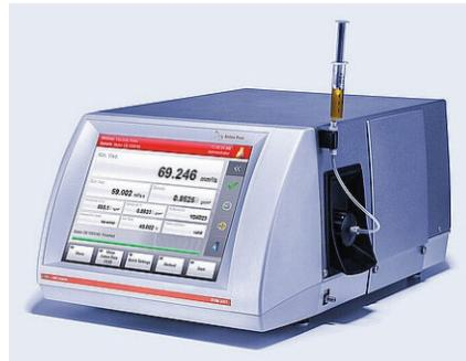
**Description of the method:** Stabinger Viscometer (SVM) is intended for measuring dynamic viscosity and density of liquid, mainly oily samples and simultaneously calculating their kinematic viscosity and other related measuring quantities. SVM is not suitable for measuring battery electrolytes.
