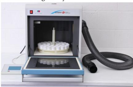
**Description of the method:** Microwave-assisted organic synthesis is a routine method used to carry out various chemical reactions in all branches of chemistry. It implies irradiation of the reaction mixture with microwaves at a frequency of 2,45 GHz, changing the temperature and reaction time. Pyrex glass cuvettes are used for reactions under normal pressure or quartz cuvettes for reactions under elevated pressure.
