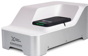
**Description of the method:** Dynamic Light Scattering (DLS) is a non-invasive method used for measuring size and size distribution of molecules and particles in submicron region, and with the latest technology, lower than 1 nm. This method is used for characterization of particles, emulsions or molecules which have been dispersed or dissolved in a liquid.
