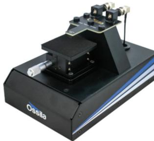
**Description of the method:** The Ossila probe for measuring sheet resistance contains four metal contacts that enable precise measurement of the resistance of very thin materials and films.
