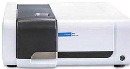
**Description of the method:** Ultraviolet-visible (UV-Vis) spectrophotometers use a light source to illuminate a sample with light across the UV to the visible wavelength range. The instruments then measure the light absorbed, transmitted, or reflected by the sample at each wavelength. From the spectrum obtained it is possible to determine the chemical or physical properties of the sample.
