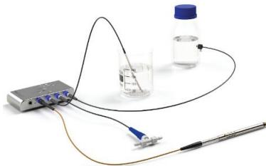
**Technical description of the device:** The compact FireSting-O<sub>2</sub> is a PC-controlled (USB) fiber-optic oxygen meter that can be combined with the complete optical oxygen sensor and optical temperature sensor portfolio, ranging from microsensors (50 µm tip) to robust probes (3 mm tip).
