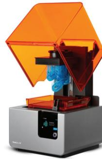
**Description of the method:** Stereolithography is a 3D printing technology that uses resin in liquid form as a starting material. The liquid resin is polymerized and cross-linked with a 405 nm wavelength laser, resulting in a solid object.
