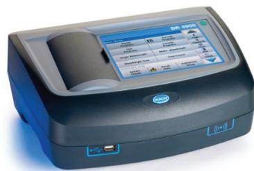
**Description of the method:** Analytical spectroscopic methods are based on measurement of the radiation amount reflected or absorbed by atomic or molecular species in the sample. When sample is exposed to the beam of light, there is a decrease in the intensity of the output radiation that is measured. This phenomenon is called light absorbance and is equal to the logarithm of the ratio of incoming and outgoing radiation.
