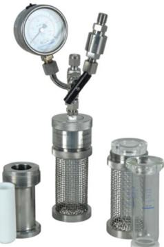
**Description of the method:** Organic synthesis is carried out in autoclaves under elevated pressure, allowing the reaction mixture to be heated to a temperature much higher than the boiling point of the solvents used. The reaction is carried out in a mini reactor of 10 to 25 ml. Glass pressure reactors ensure high acid resistance and allow visual control and process monitoring. They are used to test new chemical processes.
