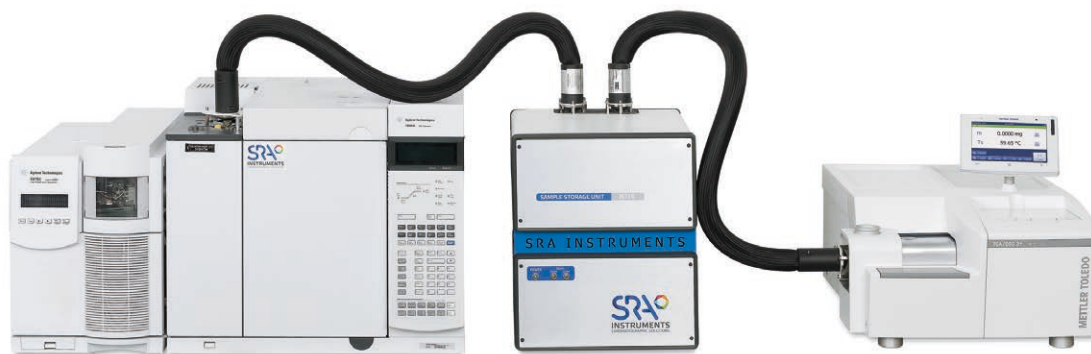
Figure 1. Right: the TGA-GC/MS system. Middle: the storage interface (IST16 or IST1). Left: the GC/MS.
