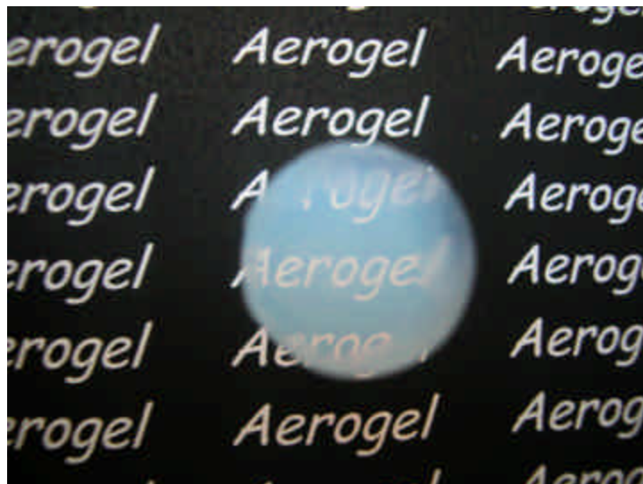
Figure 2. Photograph of a transparent, crack-free aerogel prepared in this study.
