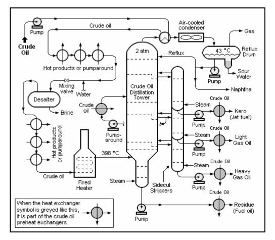
The overhead distillate fraction from the distillation column is naphtha. The fractions removed from the side of the distillation column at various points between the column top and bottom are called *sidecuts*.
