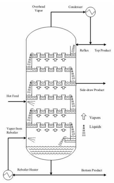
Modern crude distillation towers can process 200,000 barrels of oil per day. They can be up to 150 feet (50 meters) tall and **contain 20 to 40 fractionation trays spaced at regular intervals**. In some towers, the trays in the top section are replaced with structured packing. Before reaching the tower, **desalted oil goes through a network of preheat exchangers to a fired heater**, which brings the temperature up to about **350** °C.
