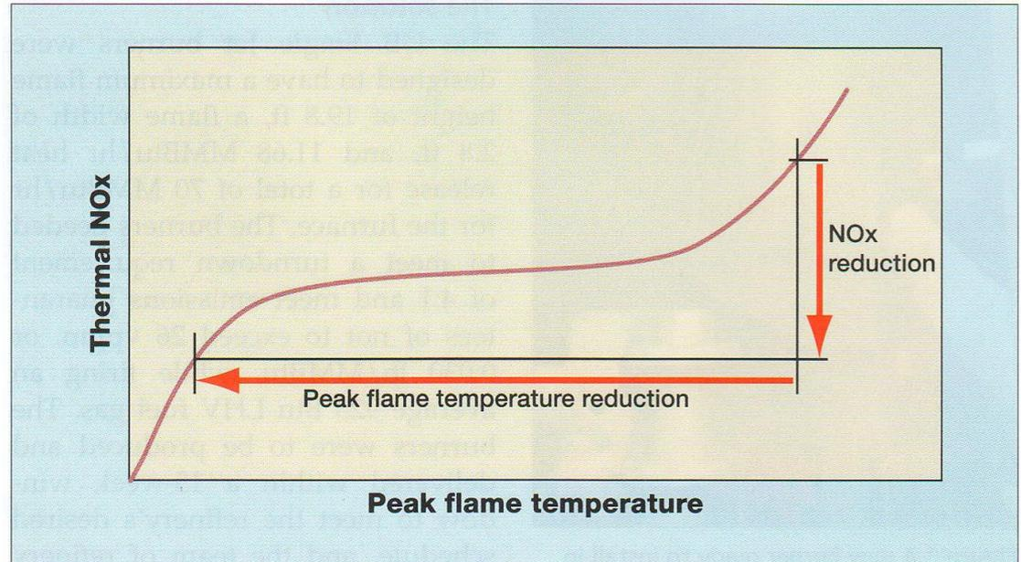
**Figure 3** Peak flame temperature versus thermal NOx production
