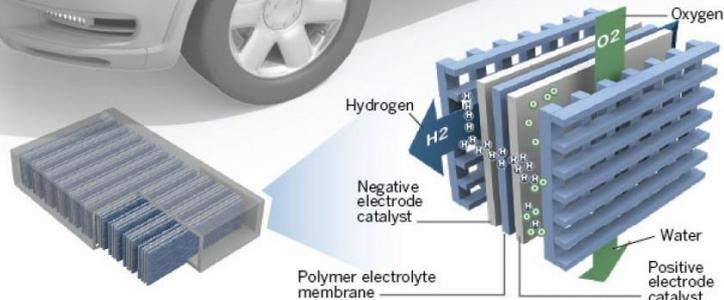
Inside each cell, hydrogen passes through a negative electrode where a catalyst strips electrons from the atoms. The electrons flow from the negative to the positive electrode, generating electricity. Electrons and hydrogen atoms travel through an electrolyte membrane to reach the positive side, where they join with oxygen to become water.
