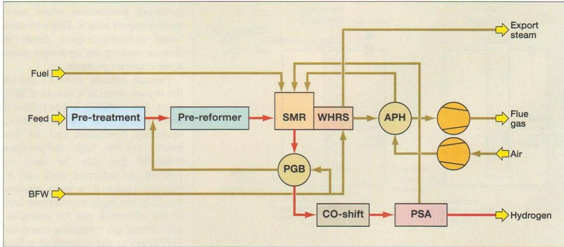
Figure 1 Typical H<sub>2</sub> SMR configuration: WHRS – waste heat recovery section, APH – air preheat, PGB – process gas boiler, PSA – pressure swing adsorption, BFW – boiler feed water
