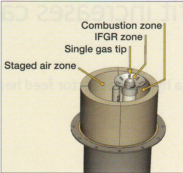
**Figure 2** Burner throat of a typical GB Single Jet burner showing the different combustion air and internal flue gas recirculation zones of the burner
