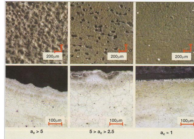
Figure 9 Overview of internal surface morphology (top pictures) and cross-sections after etching (bottom pictures) of the helical tube made in less resisting alloy after 8000 hours of operation as a function of carbon activity
