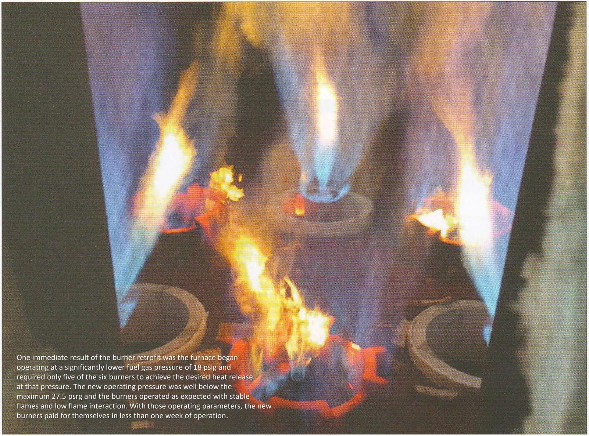
One immediate result of the burner retrofit was the furnace began operating at a significantly lower fuel gas pressure of 18 psig and required only five of the six burners to achieve the desired heat release at that pressure. The new operating pressure was well below the maximum 27.5 psig and the burners operated as expected with stable flames and low flame interaction. With those operating parameters, the new burners paid for themselves in less than one week of operation.
