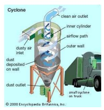
cyclone collector, for removing relatively coarse particulates from the air. Small cyclone devices are often installed to control pollution from mobile sources.
