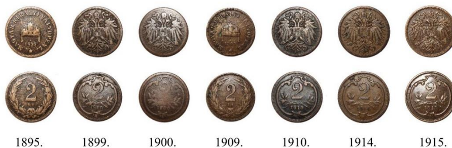
Fig. 10. Austro-Hungarian 2 Heller coins from a private collection that were subjected to EIS testing in the novel cell.
