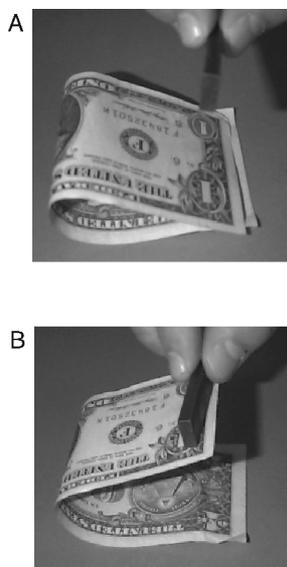
Figure 1. Magnetic inks are printed onto paper money for identification purposes. When a strong magnet is brought near a dollar bill (A), the bill is attracted to the magnet (B).
