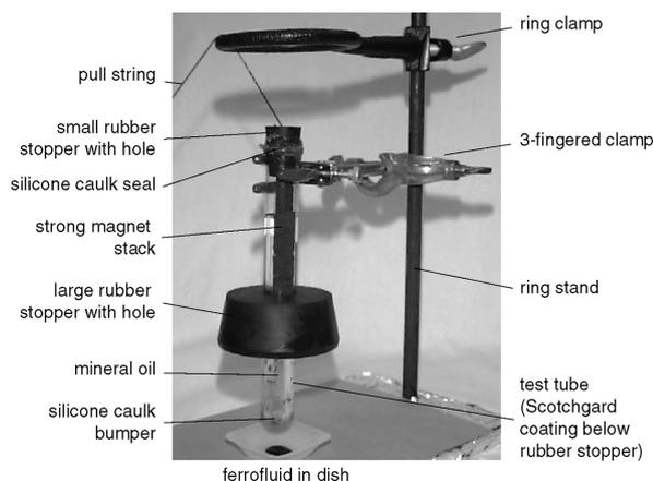
Figure 9. Construction of the "leaping ferrofluid" demonstration.
