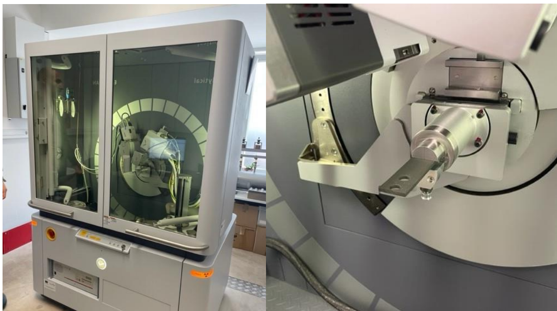
Slika 13. XRD, Panalytical Empyrean difraktometar, Malvern
