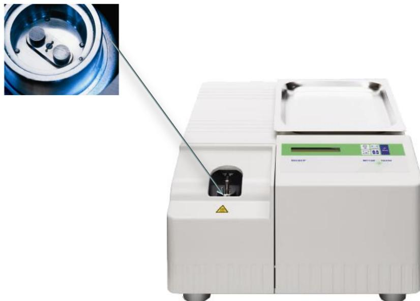
Prikaz DSC instrumenta (Mettler toledo DSC 823 e)
