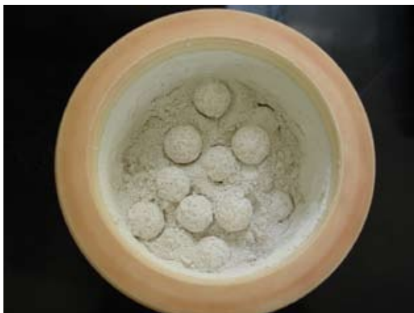
Usitnjavanje dolomita u planetarnom mlinu. Planetary ball mill comminution of dolomite.
