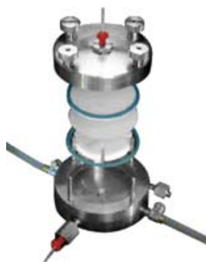
Enzimski membranski reaktor. Membrane enzyme reactor.
