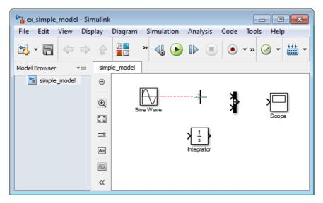
**3** Release the mouse button when the pointer is over the output port.
