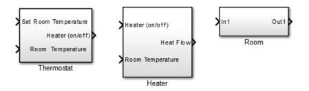
Notice the Thermostat subsystem now has a second input port. Each input port corresponds to an Inport block in the subsystem.
