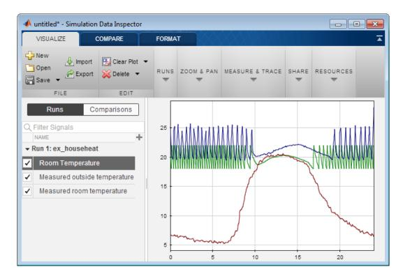
The top signal is the measured inside (room) temperature. The middle signal is the simulated room temperature. The bottom signal is the measured outside temperature.
