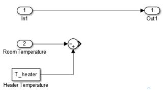
**6** Add labels to the signal lines to help trace model components to the equations and model requirements. Double-click above a signal line and enter a label.
