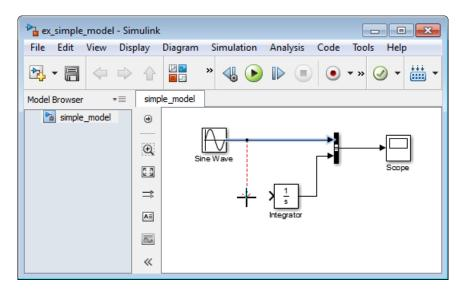
**3** Drag the cursor to the Integrator input port, and then release the mouse button.
