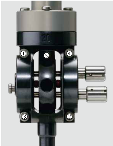
Figure 1. Installing the shear sample holder in the clamping assembly.
